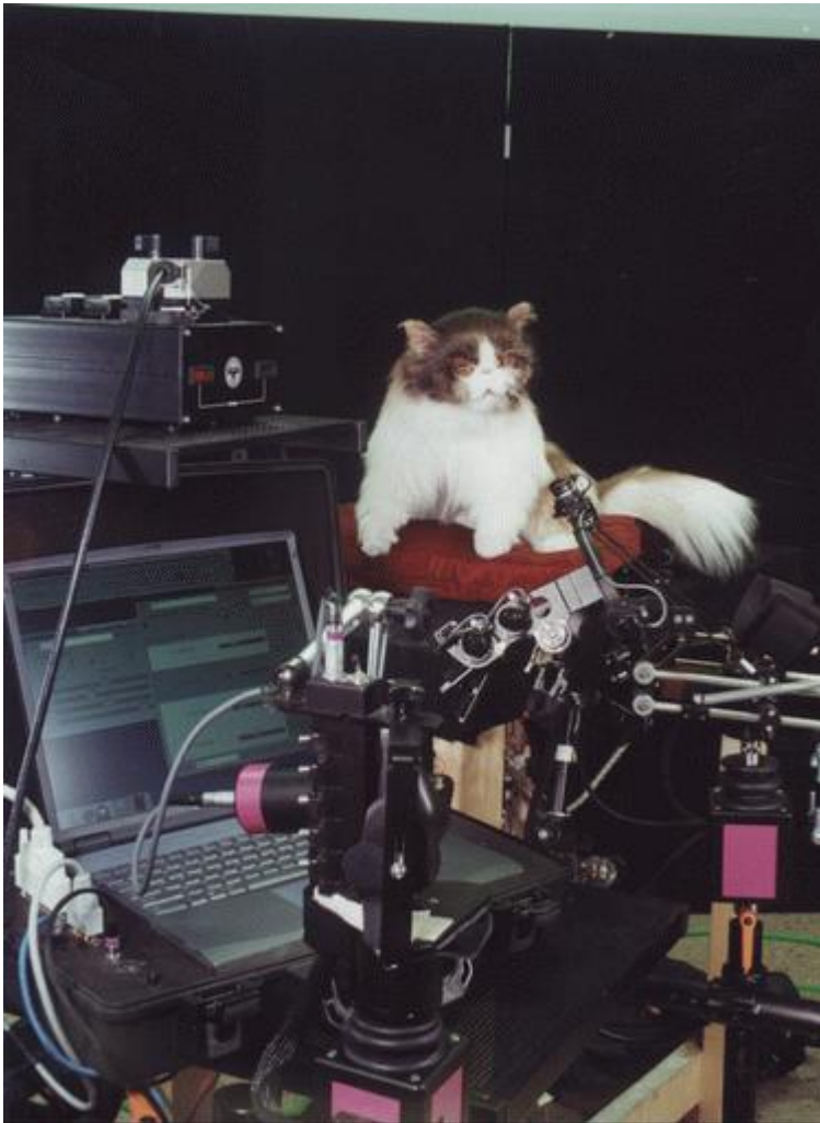
PCS setup for animatronic puppets, showing input controls and Control System laptop displaying the GUI.
