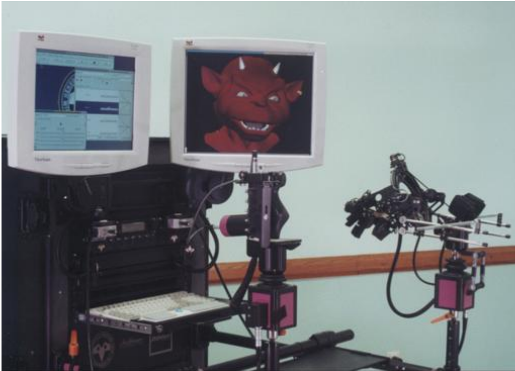
HDPs rackmount setup for 3-D CG characters showing hand controls, GUI screen and Viewer.
